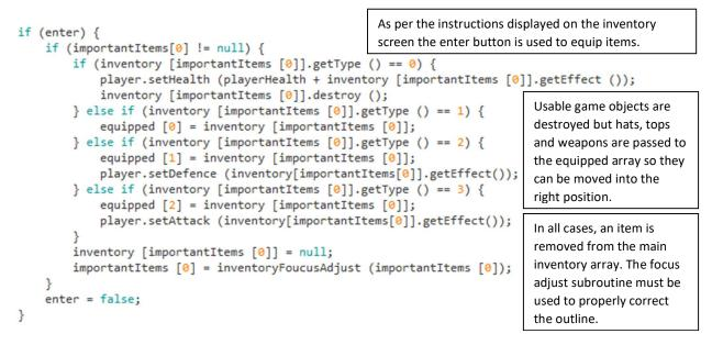
This code worked to correctly put hats, tops and weapons in the correct equipped slot. The code also adjusted the players attack and defence accurately.
