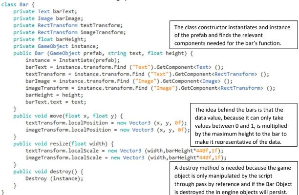
I then made a temporary adjustment to the 'Populate' subroutine to instantiate some bars and test the functionality of the subroutine.
