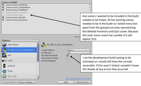
The first step to building the application was to adjust the build settings menu.
