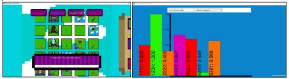
The first step in fixing this issue was determining which aspect would best fit my application. Testing the various options available I found that my application was quite close to a 4:3 ratio. I locked the scene view of the game engine to this ratio and set it as the only option for build resolutions in the build settings.
